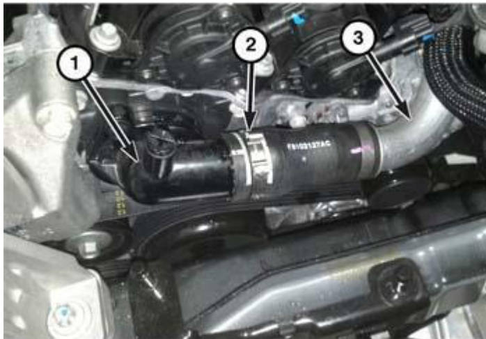
Fig. 730: Installing Thermostat Housing Courtesy of CHRYSLER GROUP, LLC
