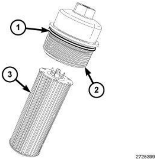
Fig. 546: O-Ring Seal, Oil Filter Cap & Oil Filter Courtesy of CHRYSLER GROUP, LLC
