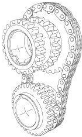
Fig. 657: Primary Chain, Idler Sprocket & Crankshaft Sprocket Courtesy of CHRYSLER GROUP, LLC
