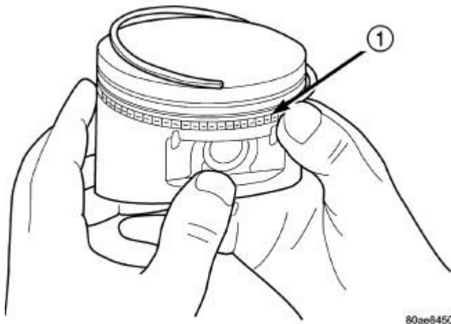
Fig. 392: Removing/Installing Piston Ring Side Rail Courtesy of CHRYSLER GROUP, LLC
