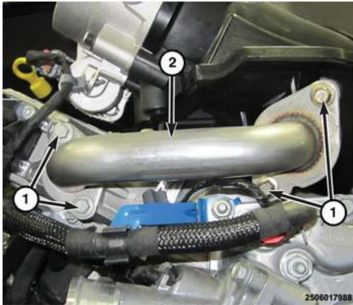
Fig. 339: Removing/Installing EGR Crossover Tube Courtesy of CHRYSLER GROUP, LLC
