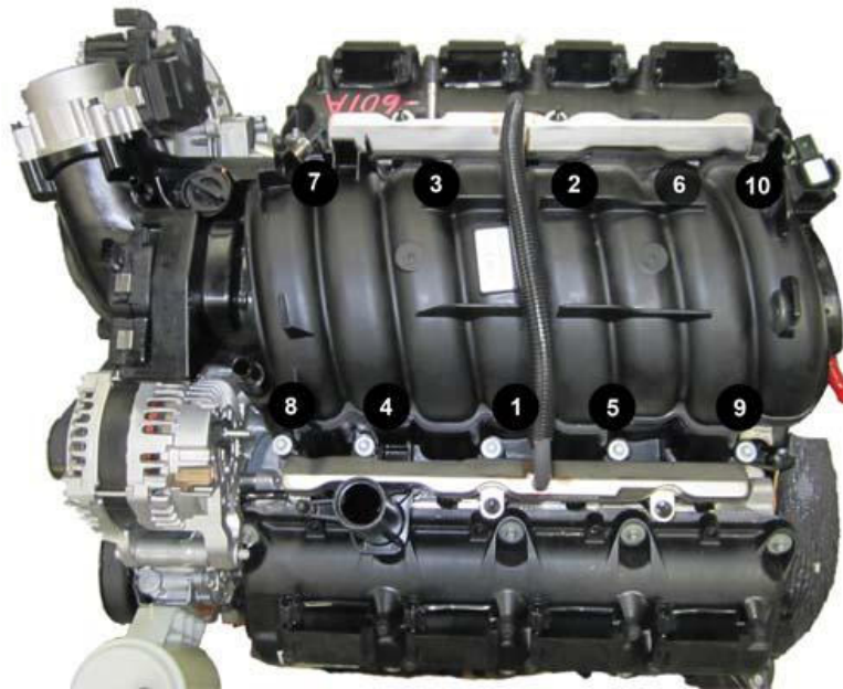
Fig. 334: Intake Manifold Removal/Installation Sequence Courtesy of CHRYSLER GROUP, LLC
