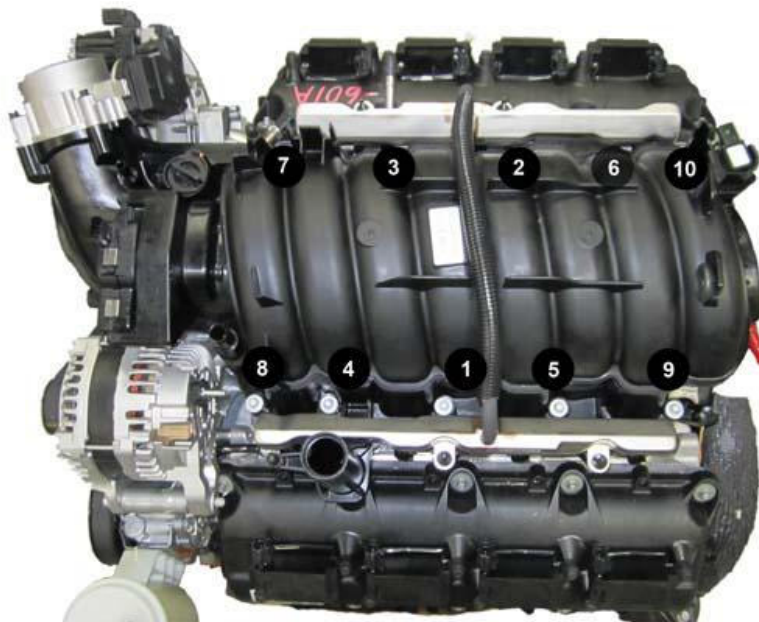
Fig. 336: Intake Manifold Removal/Installation Sequence Courtesy of CHRYSLER GROUP, LLC
