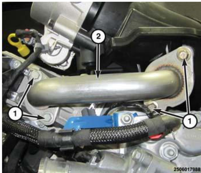
Fig. 333: Removing/Installing EGR Crossover Tube Courtesy of CHRYSLER GROUP, LLC
