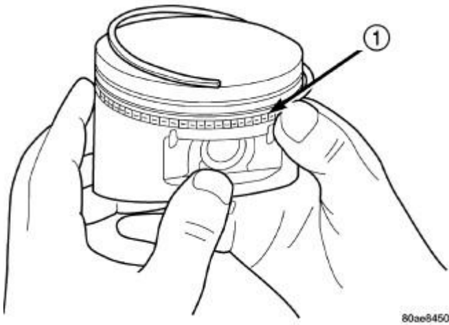
Fig. 207: Installing Piston Ring Side Rail Courtesy of CHRYSLER GROUP, LLC
