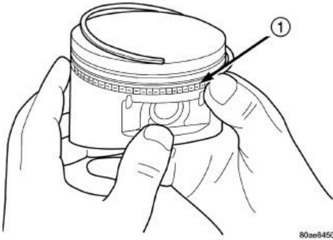
Fig. 133: Removing/Installing Piston Ring Side Rail Courtesy of CHRYSLER GROUP, LLC
