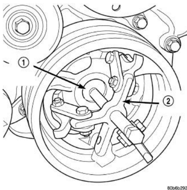
Fig. 193: Removing Crankshaft Damper Courtesy of CHRYSLER GROUP, LLC
