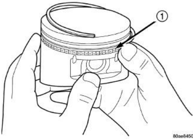
Fig. 133: Removing/Installing Piston Ring Side Rail Courtesy of CHRYSLER GROUP, LLC
