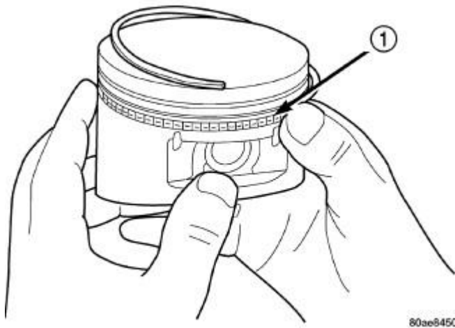
Fig. 145: Removing/Installing Piston Ring Side Rail Courtesy of CHRYSLER GROUP, LLC
