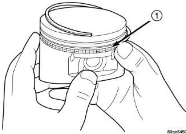
Fig. 97: Removing/Installing Piston Ring Side Rail Courtesy of CHRYSLER GROUP, LLC
