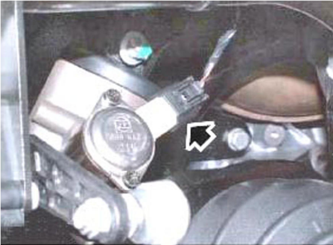
Fig. 135: Disconnecting Multiplug From Power Assisted Steering Rack Pinion Sensor Courtesy of LAND ROVER NORTH AMERICA, INC.
