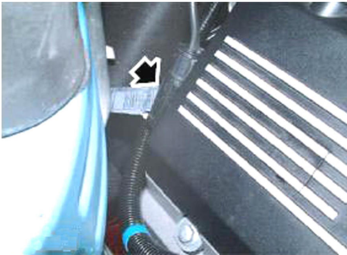
Fig. 91: Disconnecting Starter Motor Lead Multiplug Courtesy of LAND ROVER NORTH AMERICA, INC.
