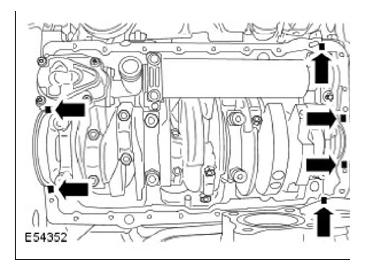
**CAUTION:** Make sure the gasket is installed correctly.
