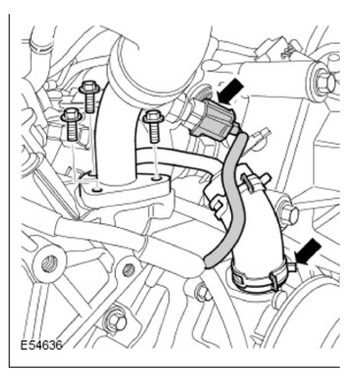
7. Remove the RH hydraulic timing chain tensioner.
