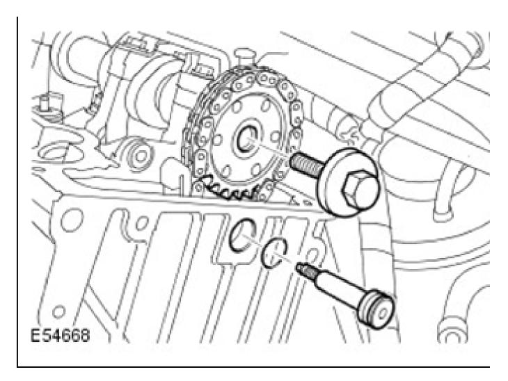
CAUTION: Working in a diagonal sequence, progressively loosen the bolts.
