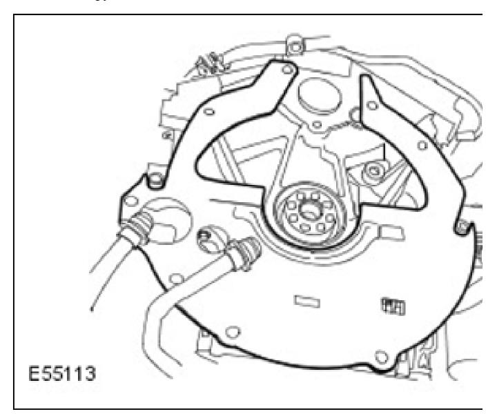
CAUTION: Care must be taken to avoid damage to the seal register and running
