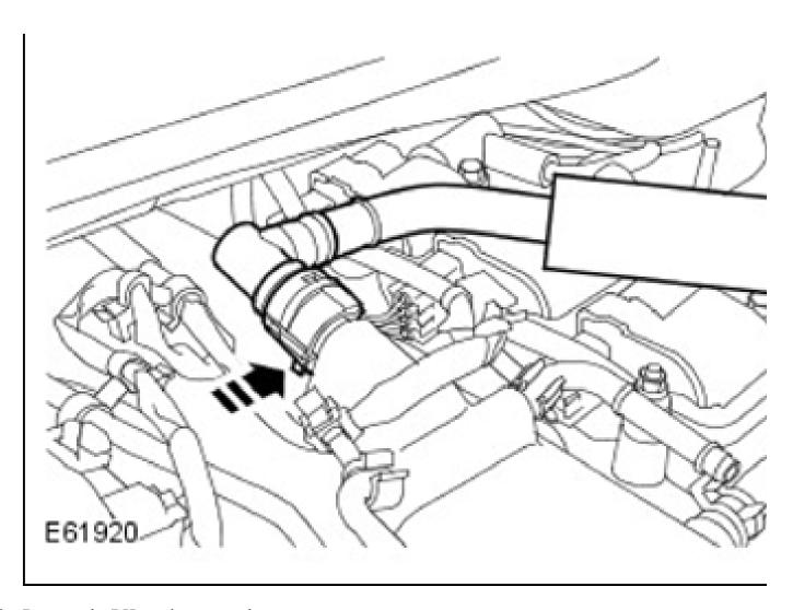
9. Remove the RH crankcase vent hose.
