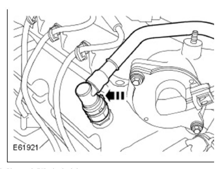
10. Disconnect the EGR valve electrical connector.
