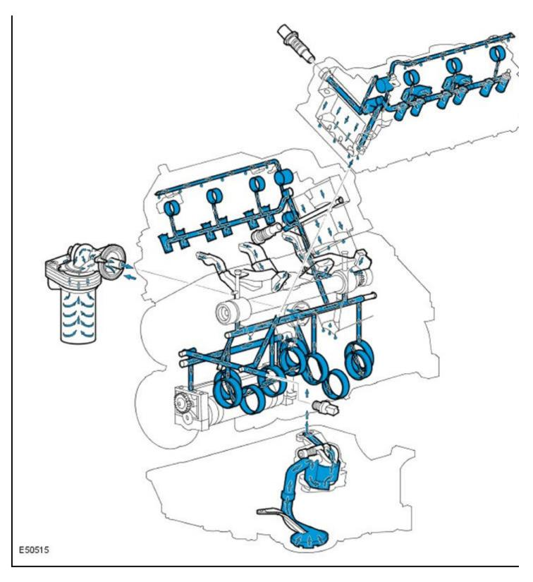
The lubrication system is of the full-flow filtration, force-fed type.
