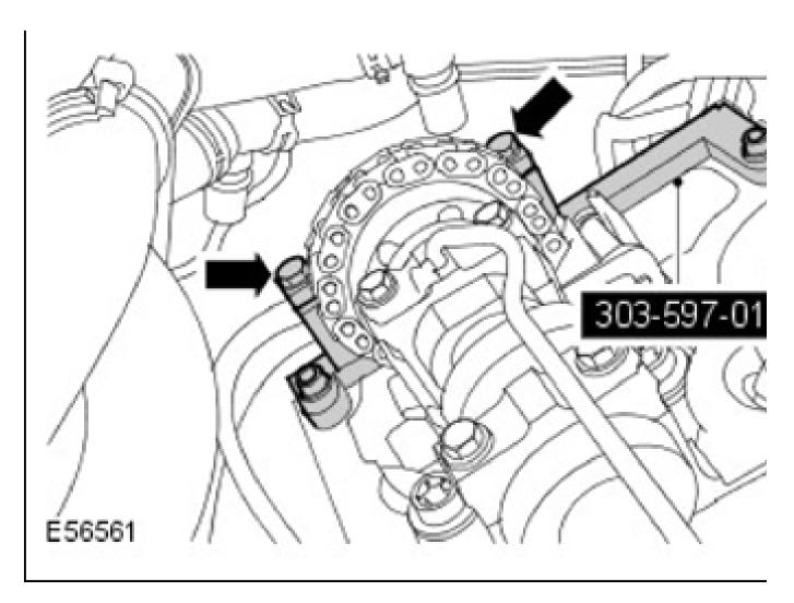
18. Using the special tool, tighten the camshaft sprocket bolt to 20 Nm (15 lb.ft), then a further 100 degrees.
