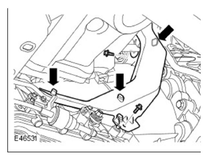
WARNING: Support the engine. The engine will fall forward when the transmission is removed.
