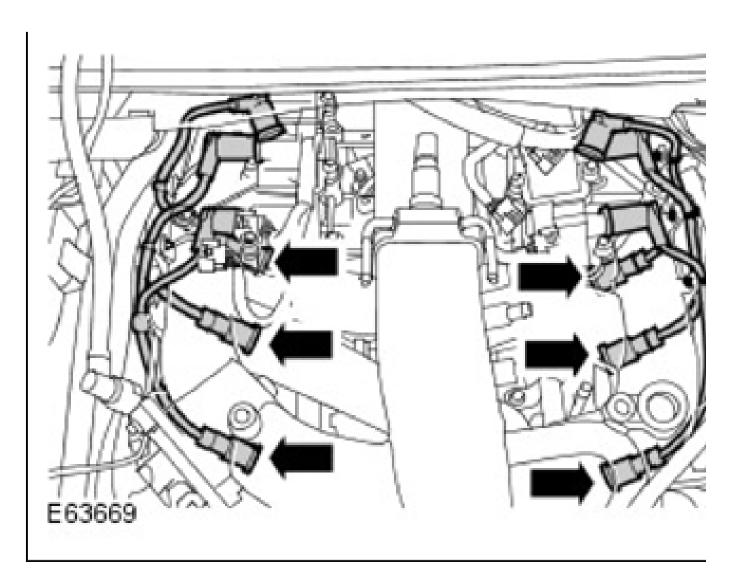
19. Position the engine wiring harness aside for access.
