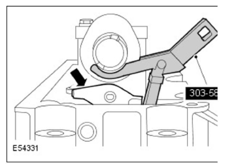
6. Rotate the engine as required to access the remaining camshaft roller followers.
