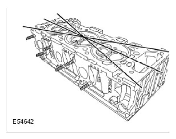
CAUTION: The head gasket must be installed over the cylinder block dowels.
