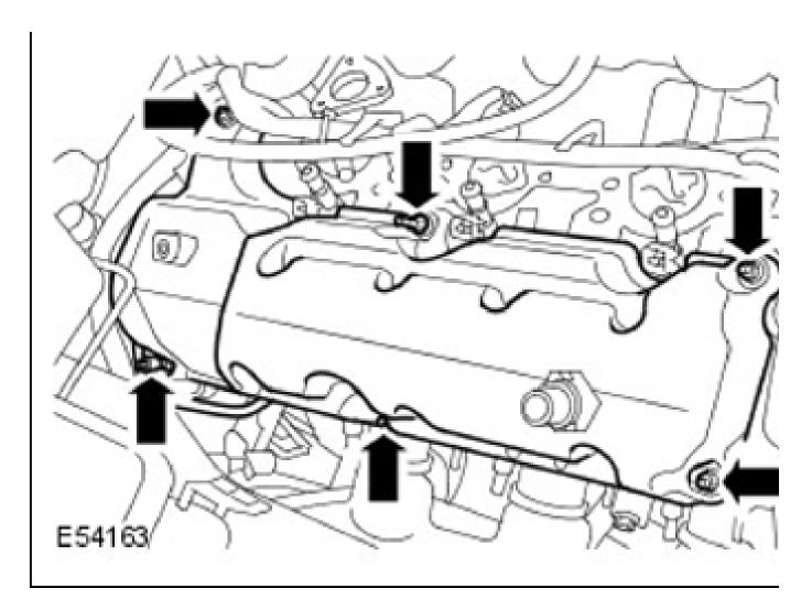
NOTE: Do not disassemble further if the component is removed for access only.
