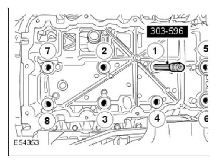
NOTE: The sealing washers are fitted to the silver coloured bolts. The silver coloured bolts are fitted in the 2 forward holes.
