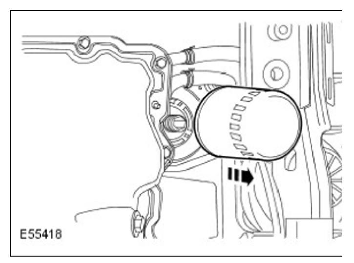
NOTE: Note the fitted position of the oil cooler assembly.
