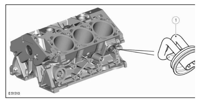
For cold climate markets an engine block heater is fitted, which is located at the front of the LH side of the cylinder block.
