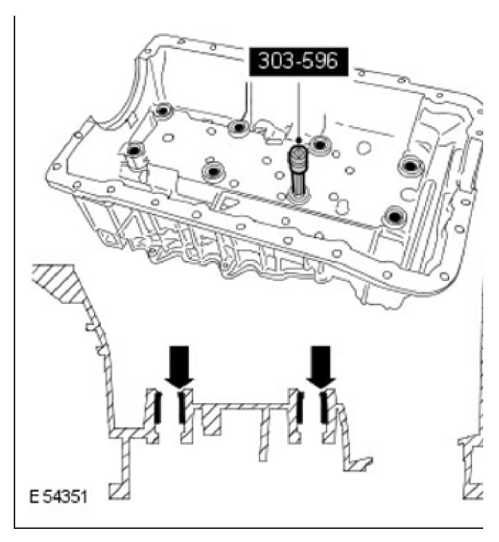
NOTE: The cradle must be installed within 20 minutes of the sealant application.
