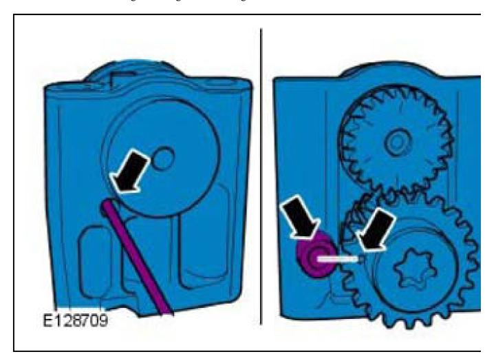
3. Rotate crankshaft clockwise until number one cylinder is at TDC and install the special tool.
