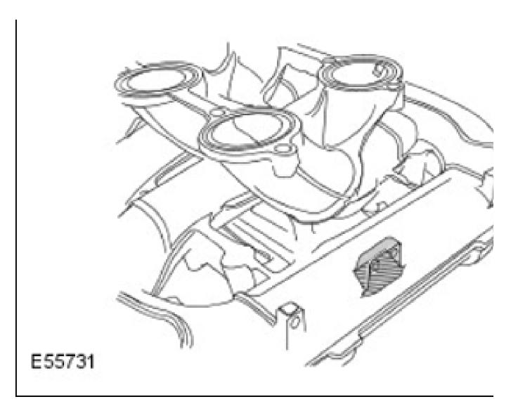
2. Early vehicles only: Remove excess material from the outside edges of the 6 intake manifold flange faces; file to within 2 mm of the gasket edge.
