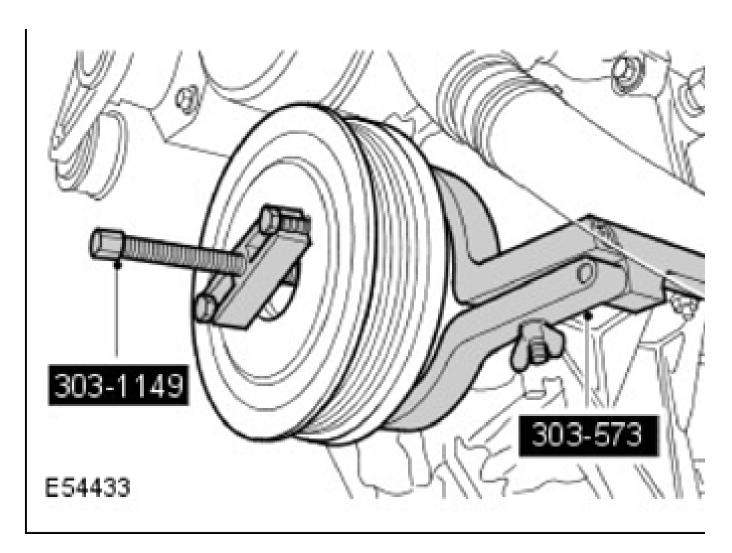
6. Using the special tool, remove the crankshaft front seal.
