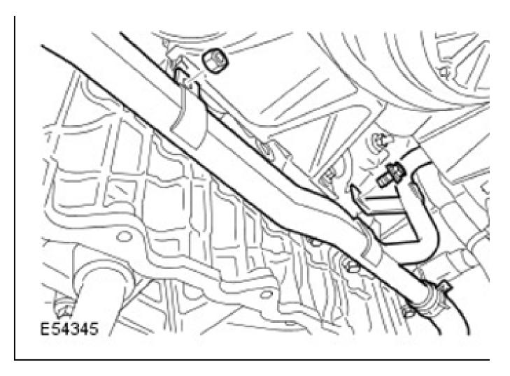
CAUTION: Before disconnecting or removing the components, make sure the area around the joint faces and connections are clean. Plug open connections to prevent contamination.
