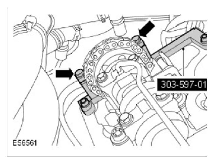
CAUTION: The RH camshaft sprocket bolt has a left hand thread.
