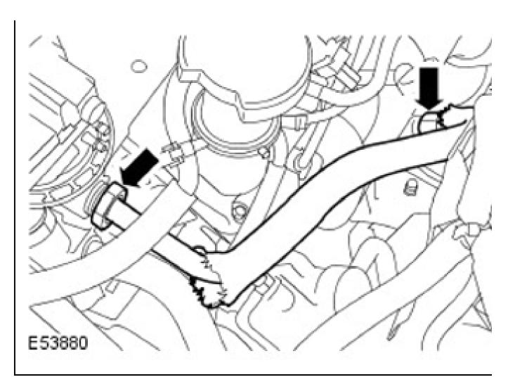
12. Disconnect the intake manifold vacuum pipe assembly.
