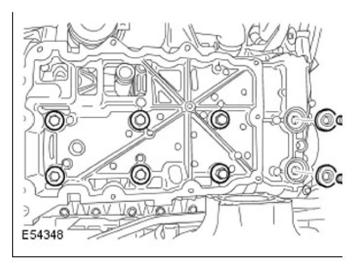
CAUTION: Failure to loosen the set screws may result in damage to the cylinder block cradle.
