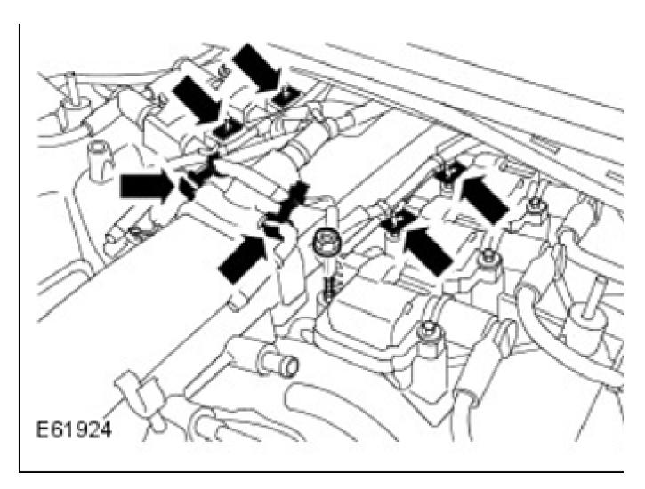
16. Disconnect the 6 coil electrical connectors.
