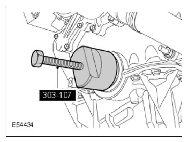
8. Check the crankshaft damper pulley and the washer for damage.
