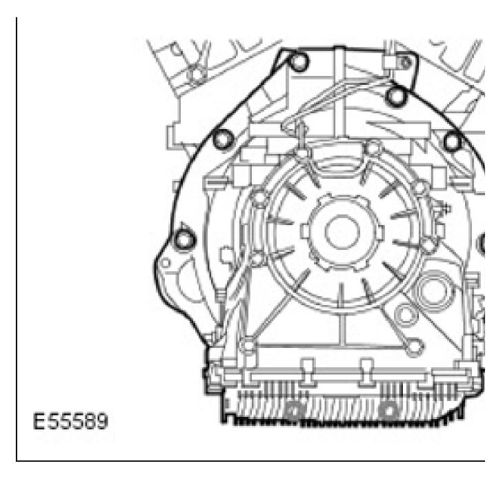
WARNING: Make sure the torque converter remains with the transmission.
