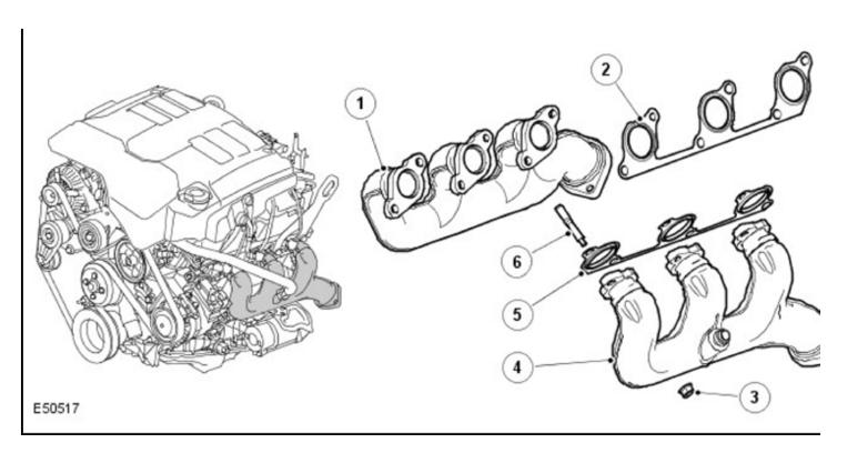
The dual wall stainless steel exhaust manifolds are unique for each cylinder bank.
