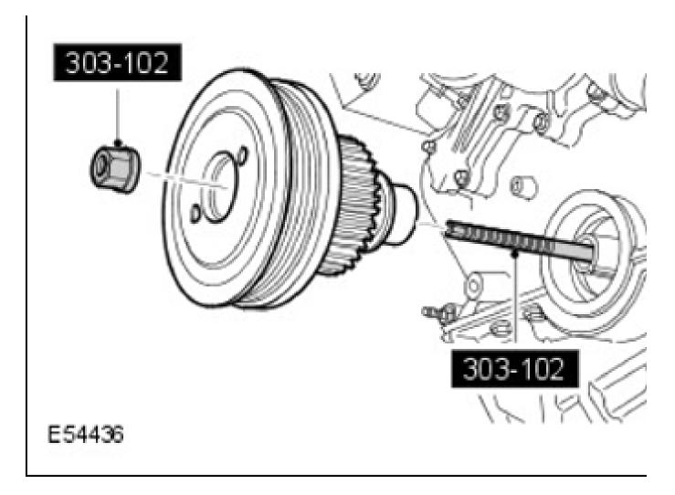
CAUTION: The screw thread in the crankshaft pulley must be cleaned out before installing a new crankshaft pulley bolt.
