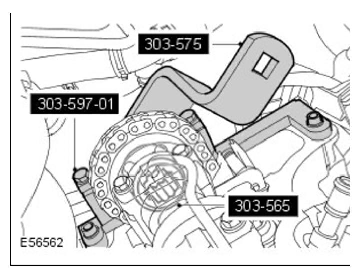
14. Loosen the special tool saddle clamp bolts.
