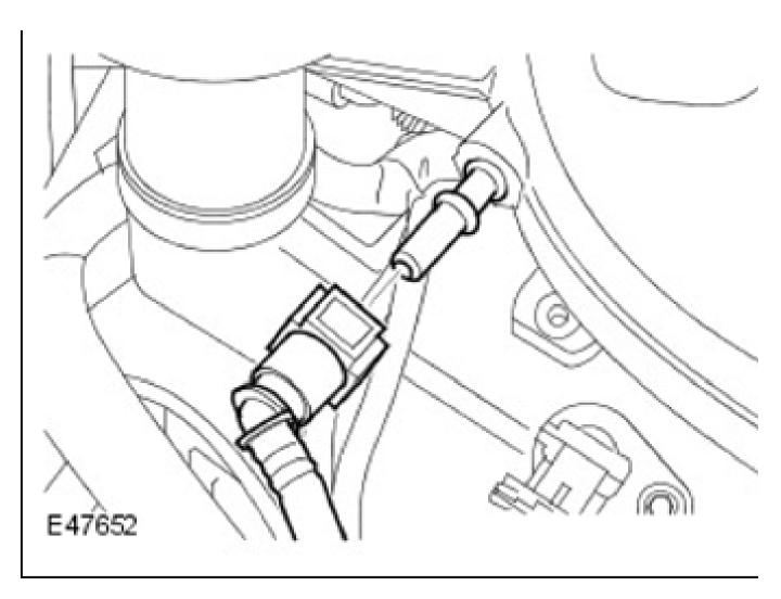
13. Disconnect the intake manifold tuning valve electrical connector.
