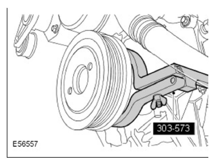
6. Install the special tool to the slot in the camshaft, the base of the special tool must remain in contact with the cylinder head. If the special tool can be passed from one side of the cylinder head to the other without resistance then the camshaft is correctly timed. Repeat the procedure on the other camshaft. If both camshafts are found to be correct, then no further action is required.
