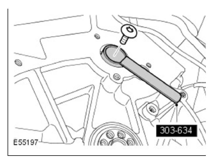
5. Remove the camshaft drive cassette LH assembly.
