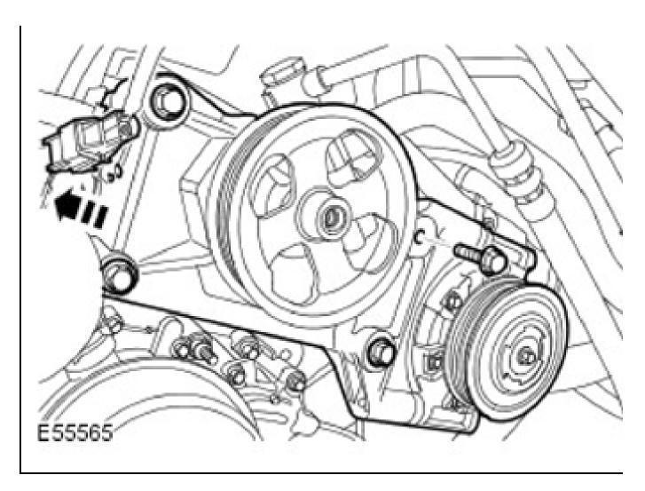
16. Disconnect the engine oil pressure (EOP) sensor electrical connector.
