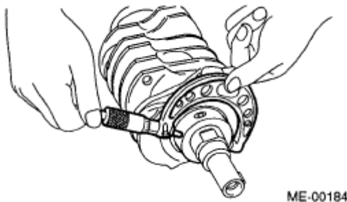
Fig. 186: Inspecting Crank Journal And Crank Pin For Wear Courtesy of SUBARU OF AMERICA, INC.
