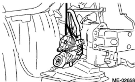
Fig. 37: Suspending Power Steering Pump Using Wire Courtesy of SUBARU OF AMERICA, INC.
