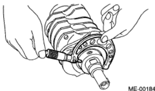
Fig. 228: Checking Crank Journal Courtesy of SUBARU OF AMERICA, INC.
