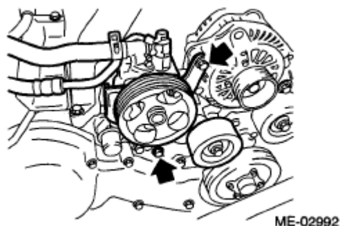
Fig. 34: Identifying Power Steering Pump Bracket Mounting Bolts Courtesy of SUBARU OF AMERICA, INC.
