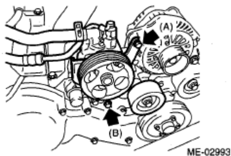
Fig. 38: Locating Power Steering Pump Bracket Bolts Courtesy of SUBARU OF AMERICA, INC.
