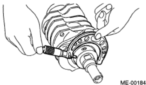
Fig. 175: Checking Crank Journal And Crank Pin
