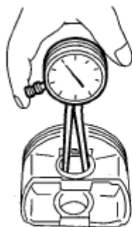
Fig. 163: Checking Clearance Between Piston Pin And Hole In Piston
