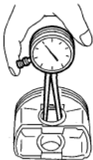
Fig. 165: Checking Clearance Of Piston Courtesy of SUBARU OF AMERICA, INC.
