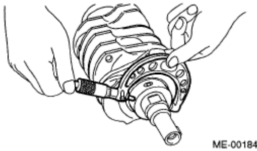
Fig. 177: Inspecting Crank Journal And Crank Pin Courtesy of SUBARU OF AMERICA, INC.
