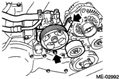
Fig. 23: Locating Power Steering Pump Bracket Bolts Courtesy of SUBARU OF AMERICA, INC.
