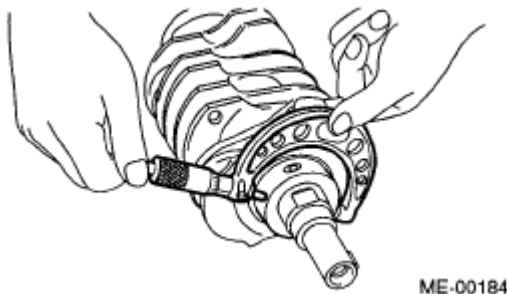
Fig. 278: Checking Crank Journal And Crank Pin For Wear Courtesy of SUBARU OF AMERICA, INC.
