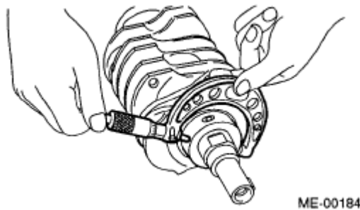
Fig. 283: Measuring Crank Journal Cylindricity Courtesy of SUBARU OF AMERICA, INC.
