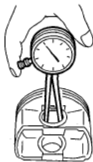
Fig. 273: Measuring Cylinder Inner Diameter Boring Limit Courtesy of SUBARU OF AMERICA, INC.
