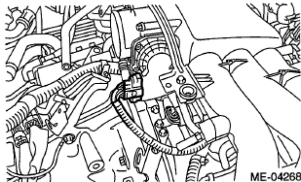
Fig. 48: Identifying Throttle Body Connector Courtesy of SUBARU OF AMERICA, INC.
