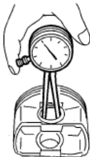
Fig. 267: Checking Clearance Between Piston Pin Hole And Piston Pin (1 Of 2) Courtesy of SUBARU OF AMERICA, INC.
