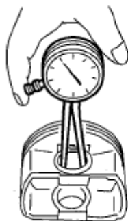
Fig. 266: Checking Clearance Between Piston Pin Hole And Piston Pin (1 Of 2) Courtesy of SUBARU OF AMERICA, INC.
