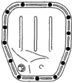
Fig. 221: Identifying Oil Pan Mounting Bolts
