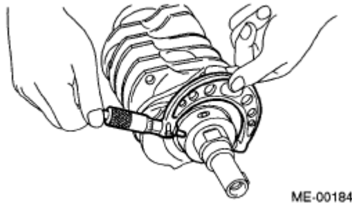
Fig. 268: Checking Crank Journal And Crank Pin Diameter Courtesy of SUBARU OF AMERICA, INC.
