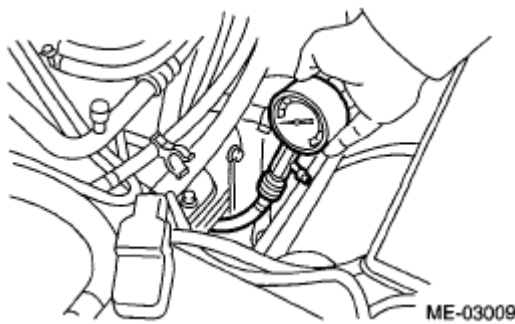
Fig. 8: Installing Compression Gauge To Spark Plug Hole Courtesy of SUBARU OF AMERICA, INC.
