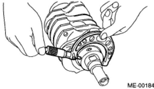
Fig. 271: Checking Crank Journal And Crank Pin For Wear Courtesy of SUBARU OF AMERICA, INC.
