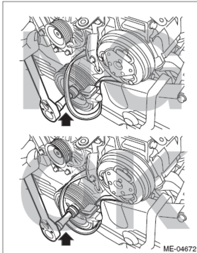
Fig. 84: Identifying Proper And Improper Placing Of Tool On Crank Pulley Bolt Courtesy of SUBARU OF AMERICA, INC.
