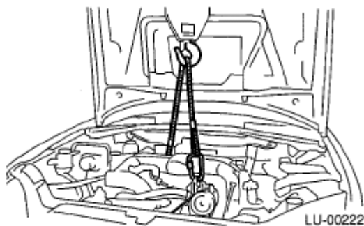
Fig. 63: Supporting Engine With Lifting Device And Wire Ropes Courtesy of SUBARU OF AMERICA, INC.
