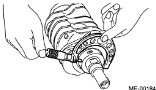
Fig. 275: Inspecting Crank Journal And Crank Pin For Wear Courtesy of SUBARU OF AMERICA, INC.
