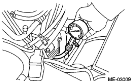
Fig. 8: Reading Compression Gauge Value Installed On Spark Plug Courtesy of SUBARU OF AMERICA, INC.
