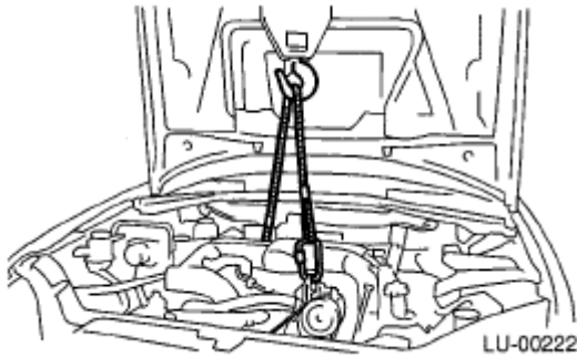
Fig. 55: Identifying Engine With Lifting Device And Wire Ropes Courtesy of SUBARU OF AMERICA, INC.
