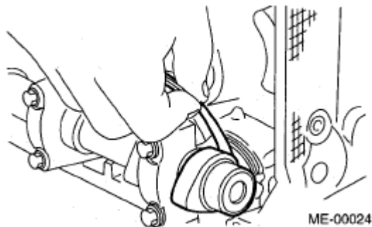
Fig. 25: Measuring Valve Clearances Courtesy of SUBARU OF AMERICA, INC.
