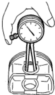
Fig. 242: Checking Clearance Between Piston Pin Hole Courtesy of SUBARU OF AMERICA, INC.
