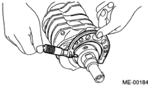
Fig. 254: Inspecting Crank Journal And Crank Pin For Wear Courtesy of SUBARU OF AMERICA, INC.
