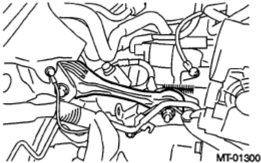
Fig. 44: Removing Pitching Stopper Courtesy of SUBARU OF AMERICA, INC.
