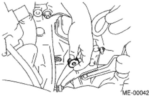
Fig. 42: Removing Plug Using Hexagon Wrench Courtesy of SUBARU OF AMERICA, INC.
