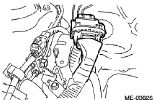
Fig. 62: Identifying Engine Harness Connectors Courtesy of SUBARU OF AMERICA, INC.
