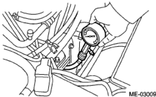
Fig. 8: Measuring Cylinder Compression Courtesy of SUBARU OF AMERICA, INC.
