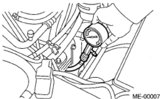
Fig. 7: Checking Compression Using Compression Gauge
