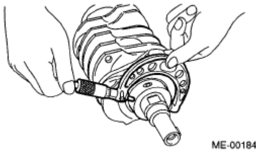
Fig. 304: Inspecting Crank Journal And Crank Pin Courtesy of SUBARU OF AMERICA, INC.
