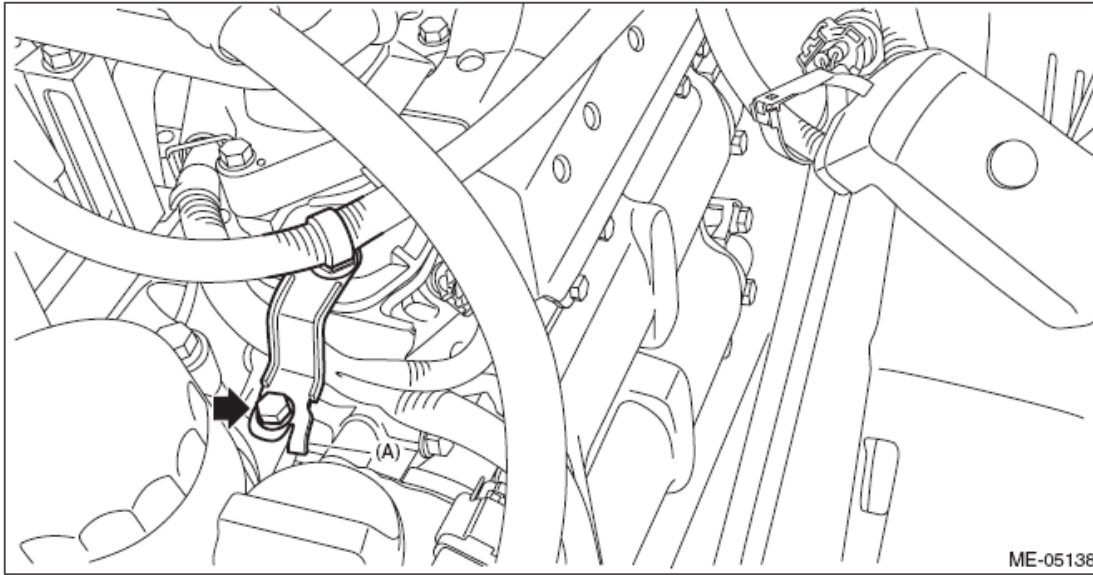
Fig. 73: Locating Chain Cover Generator Cord Stay Mounting Bolt Courtesy of SUBARU OF AMERICA, INC.
