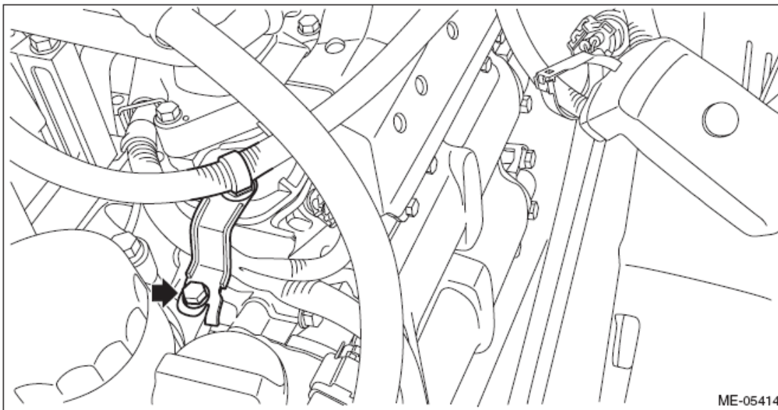
Fig. 41: Locating Generator Cord Stay Bolt Courtesy of SUBARU OF AMERICA, INC.
