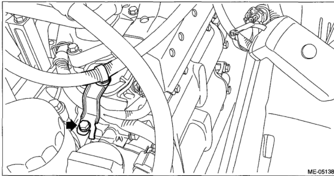
Fig. 73: Locating Generator Cord Stay Bolt Courtesy of SUBARU OF AMERICA, INC.
