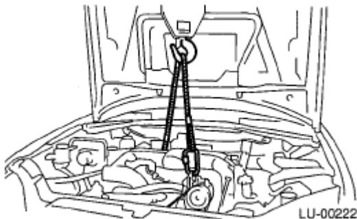
Fig. 44: Lifting Engine Away From Engine Compartment Courtesy of SUBARU OF AMERICA, INC.
