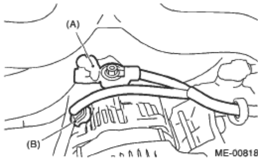
(A) Terminals (B) Generator connector
