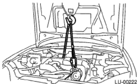
Fig. 54: Supporting Engine With Lifting Device And Wire Ropes
