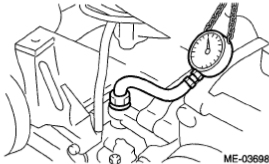
Fig. 13: Measuring Oil Pressure Courtesy of SUBARU OF AMERICA, INC.
