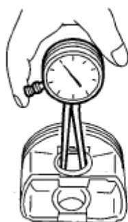
Fig. 191: Checking Piston Pin Hole Courtesy of SUBARU OF AMERICA, INC.
