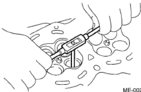
Fig. 135: Reaming Inside Of Valve Guide Using ST Courtesy of SUBARU OF AMERICA, INC.
