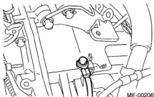
Fig. 24: Identifying Engine Ground Cable Courtesy of SUBARU OF AMERICA, INC.
