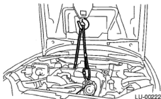
Fig. 40: Supporting Engine With Lifting Device And Wire Ropes Courtesy of SUBARU OF AMERICA, INC.
