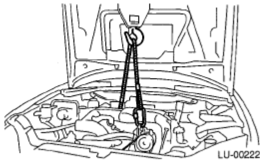
Fig. 64: Supporting Engine With Lifting Device And Wire Ropes Courtesy of SUBARU OF AMERICA, INC.
