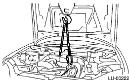
Fig. 71: Supporting Engine With Lifting Device And Wire Ropes Courtesy of SUBARU OF AMERICA, INC.
