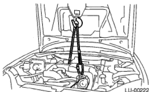
Fig. 53: Supporting Engine With Lifting Device And Wire Ropes Courtesy of SUBARU OF AMERICA, INC.
