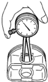
Fig. 231: Checking Clearance Between Piston Pin And Hole In Piston Courtesy of SUBARU OF AMERICA, INC.
