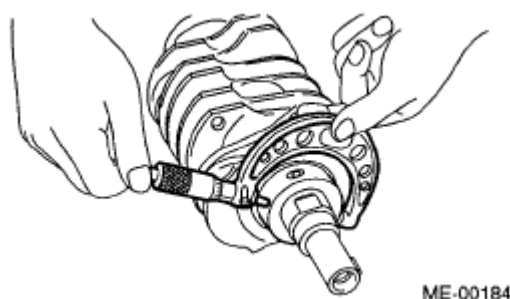
Fig. 243: Inspecting Crank Journal And Crank Pin Courtesy of SUBARU OF AMERICA, INC.
