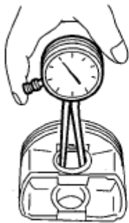
Fig. 202: Measuring Piston Hole Diameter Courtesy of SUBARU OF AMERICA, INC.
