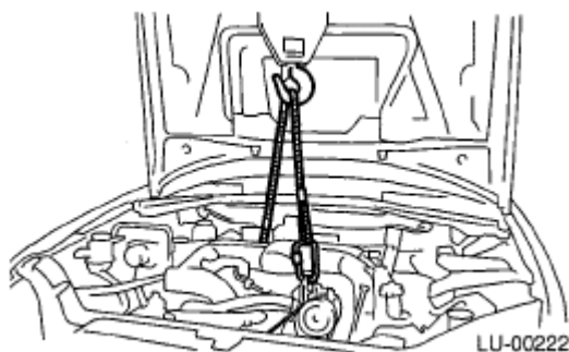
Fig. 45: Supporting Engine With Lifting Device And Wire Ropes Courtesy of SUBARU OF AMERICA, INC.
