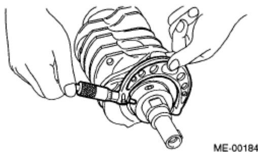
Fig. 203: Inspecting Crank Journal And Crank Pin Courtesy of SUBARU OF AMERICA, INC.
