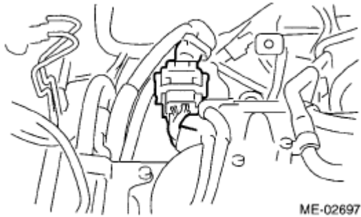
Fig. 206: Identifying Engine Harness Connector
