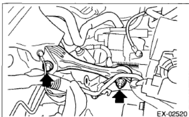
Fig. 39: Locating Pitching Stopper Bolt And Nut Courtesy of SUBARU OF AMERICA, INC.
