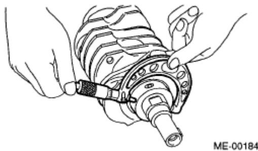
Fig. 241: Measuring Crank Journal Courtesy of SUBARU OF AMERICA, INC.
