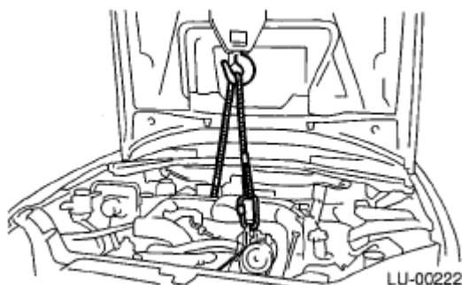
Fig. 47: Identifying Lifting Device And Wire Ropes Courtesy of SUBARU OF AMERICA, INC.
