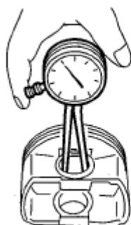
Fig. 226: Measuring Piston Hole Diameter Courtesy of SUBARU OF AMERICA, INC.
