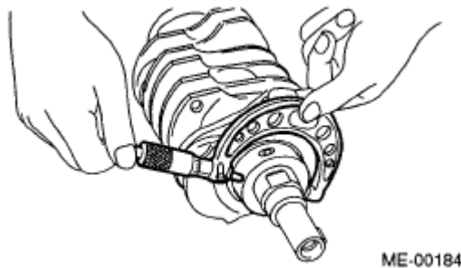
Fig. 212: Inspecting Crank Journal And Crank Pin Courtesy of SUBARU OF AMERICA, INC.
