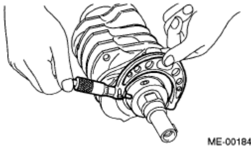
Fig. 247: Checking Crank Journal And Crank Pin Courtesy of SUBARU OF AMERICA, INC.
