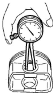
Fig. 235: Checking Clearance Between Piston Pin And Hole In Piston Courtesy of SUBARU OF AMERICA, INC.
