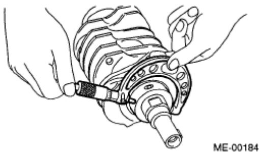
Fig. 211: Inspecting Crank Journal And Crank Pin For Wear Courtesy of SUBARU OF AMERICA, INC.
