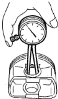
Fig. 197: Measuring Inner Diameter Of Piston Hole
