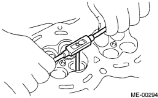
Fig. 141: Reaming Inside Of Valve Guide
