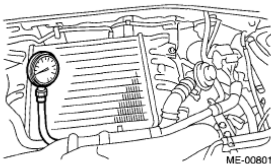
Fig. 8: Checking Intake Manifold Vacuum Pressure
