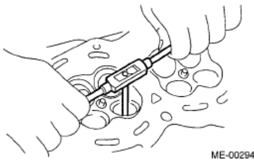
Fig. 143: Reaming Inside Of Valve Guide Using ST Courtesy of SUBARU OF AMERICA, INC.
