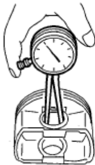
Fig. 291: Checking Clearance Between Piston Pin And Hole In Piston Courtesy of SUBARU OF AMERICA, INC.
