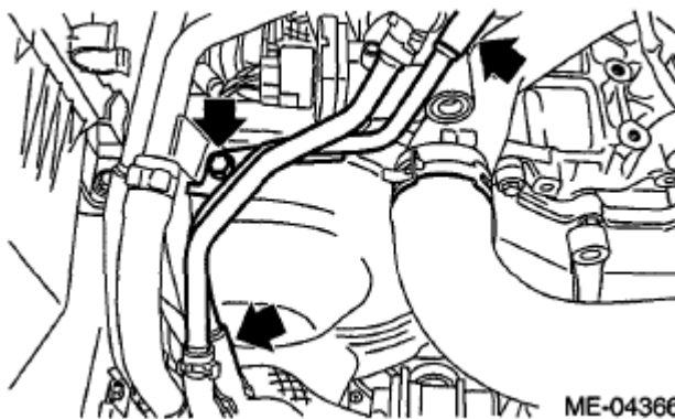
Fig. 111: Locating Vacuum Hose And Blow-By Pipe Bolt Courtesy of SUBARU OF AMERICA, INC.
