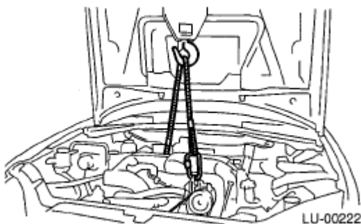
Fig. 81: Supporting Engine With Lifting Device And Wire Ropes
