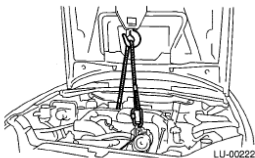
Fig. 74: Supporting Engine With Lifting Device And Wire Ropes Courtesy of SUBARU OF AMERICA, INC.
