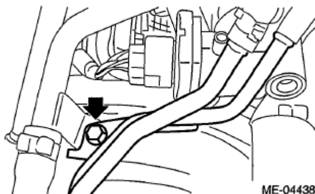
Fig. 118: Locating Blow-By Pipe Bolt Courtesy of SUBARU OF AMERICA, INC.
