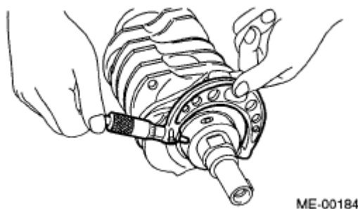
Fig. 303: Inspecting Crank Journal And Crank Pin Courtesy of SUBARU OF AMERICA, INC.
